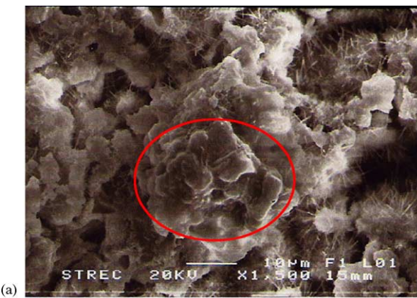
Fig. 7. (a) SEM photographs of SW4-S25-L04 at the age of 7 days focusing on hexagonal-plate morphology of hydrated calcium aluminate/ferrite; (b) EDS spectrum pointing at hexagonal-plate structure to investigate arsenic immobilization potential.
